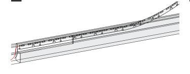
2 Solder connecting 'wire tails' to terminals for connection to power supply, or for 'bridging wires' for linking of strip segments. Always ensure positive-positive and negative-negative connection.
