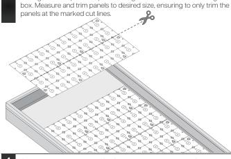
Arrange matrix spectrum panels in a grid-like fashion within the light
