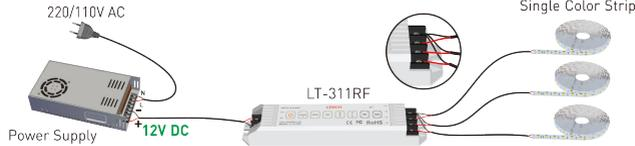
4.2 Power repeater can be added to expand power when the power is not enough. Constant current power repeater also can be added if control the high power LED at the same time.
